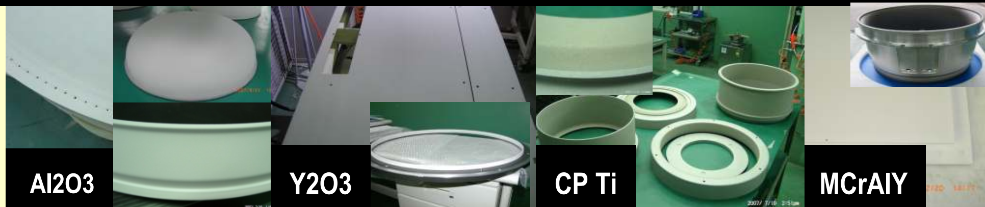
Robotic Spraying Protective Coating on 12" wafer vacuum Chamber parts
